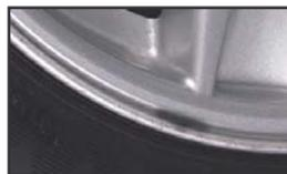
*Corrosion caused by uncoated lead weights*
